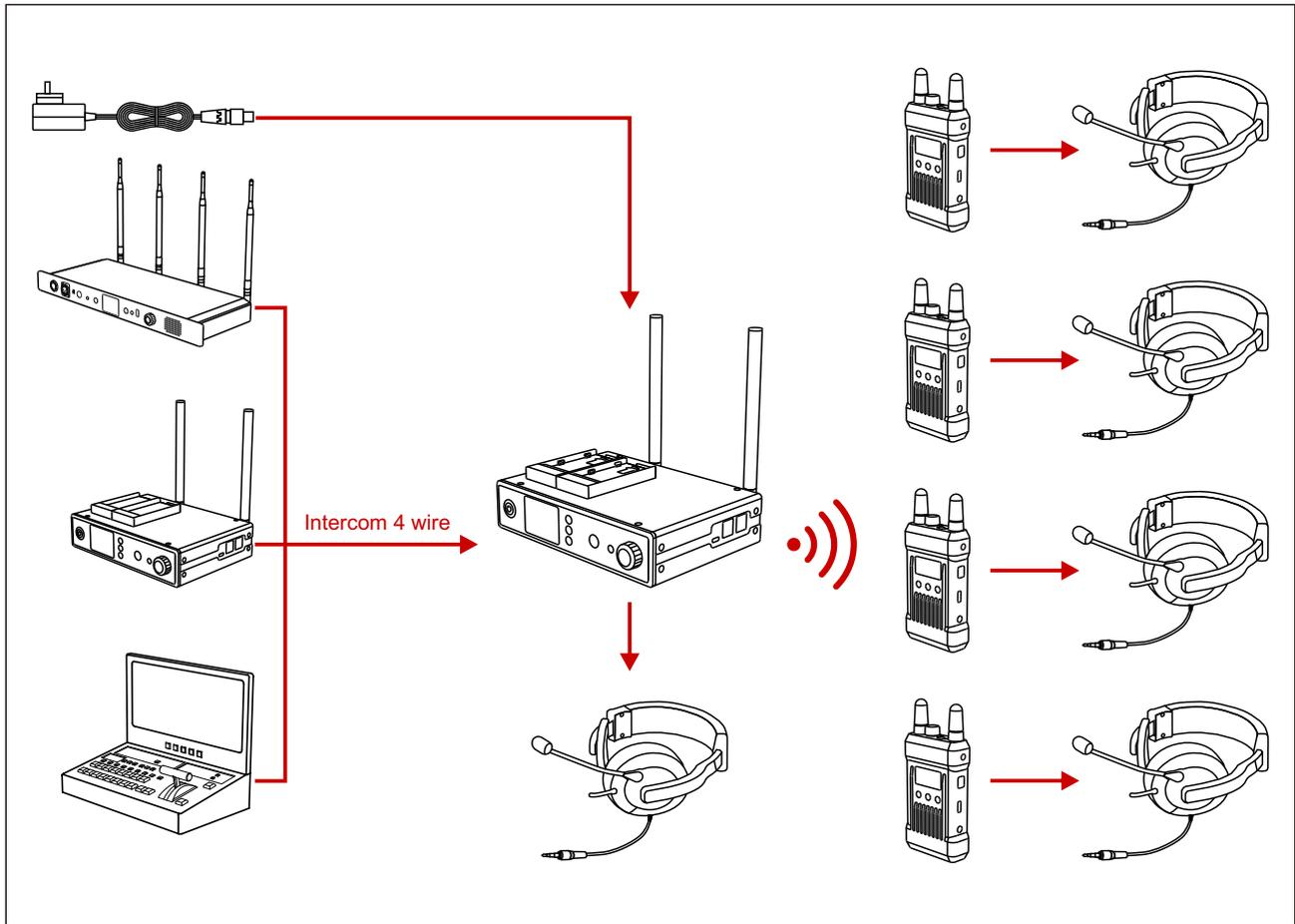
The base station of this wireless full-duplex intercom system supports 4 beltacks. The base station and the beltacks support dynamic and electret mics. They could be switched by selecting on the menu for different applications. The 4-pin audio interface on the base station enables the device to connect with other audio systems, which can increase the quantity of beltacks and also the wireless communication range.
